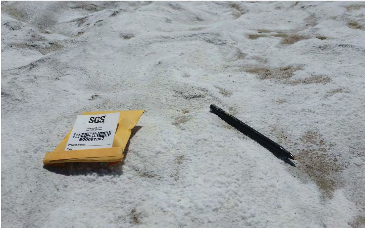
Photo 9.4. Typical sample of salt encrustation. (Sample B00067367)
