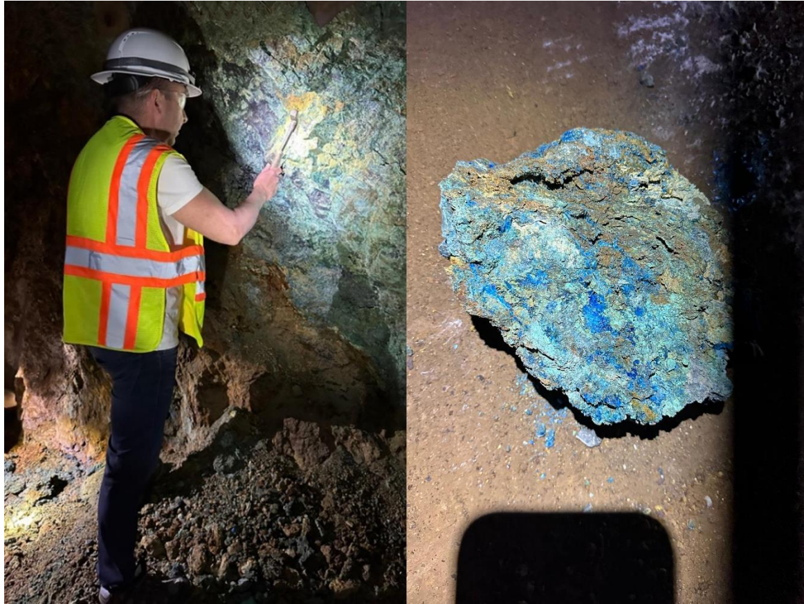
Photo 1: CEO, Warwick Smith, collects rock chip samples from Madison underground (left); high-grade copper associated with chalcantite and chalcocite from the Madison underground workings (right)
