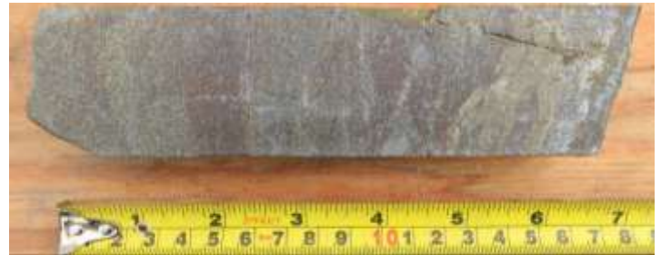
Figure 3: Banded sphalerite-pyrite-chalcopyrite-barite in hole CMR23-155, Southwall Zone 1.
