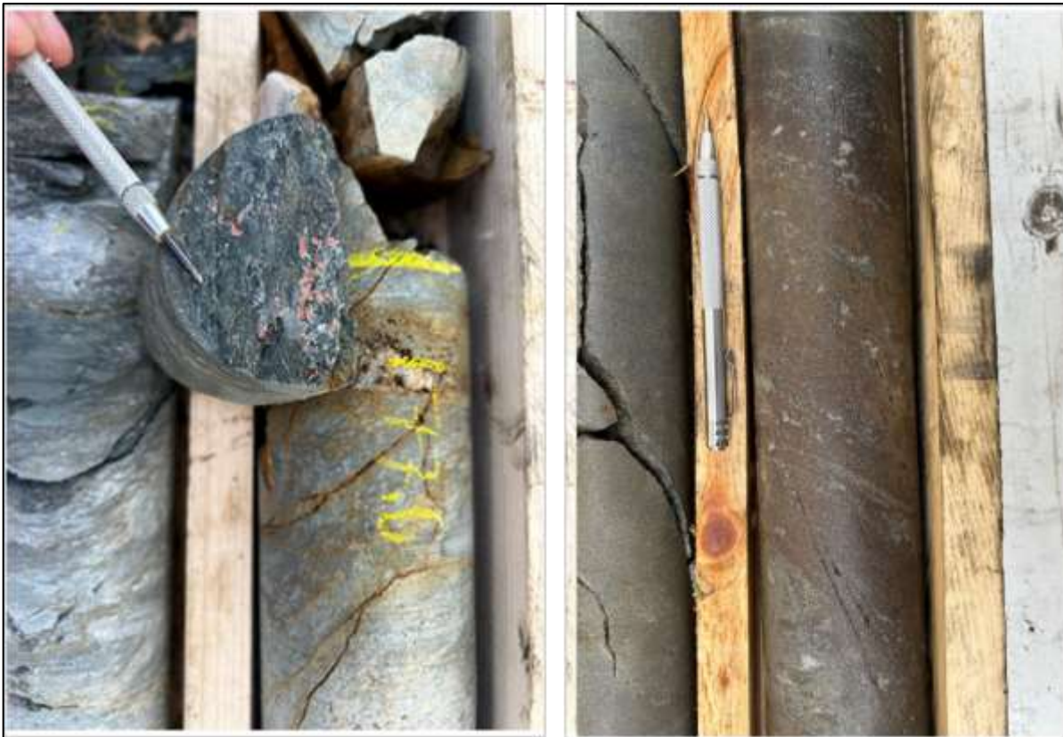
Plate 1: (left) Native copper in drillhole CMR23-152 at 177.6 m downhole (Southwall Zone 1).
