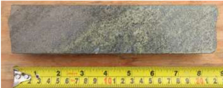
Figure 2: Massive chalcopyrite-pyrrhotite-pyrite in directional hole CMR23-157-01, Lower Southwall Zone 2-3.
