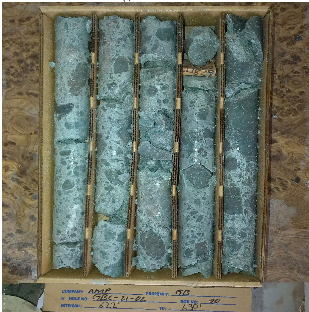
Image 1. Breccia with Andesite Clasts in a Clay Gouge Matrix
