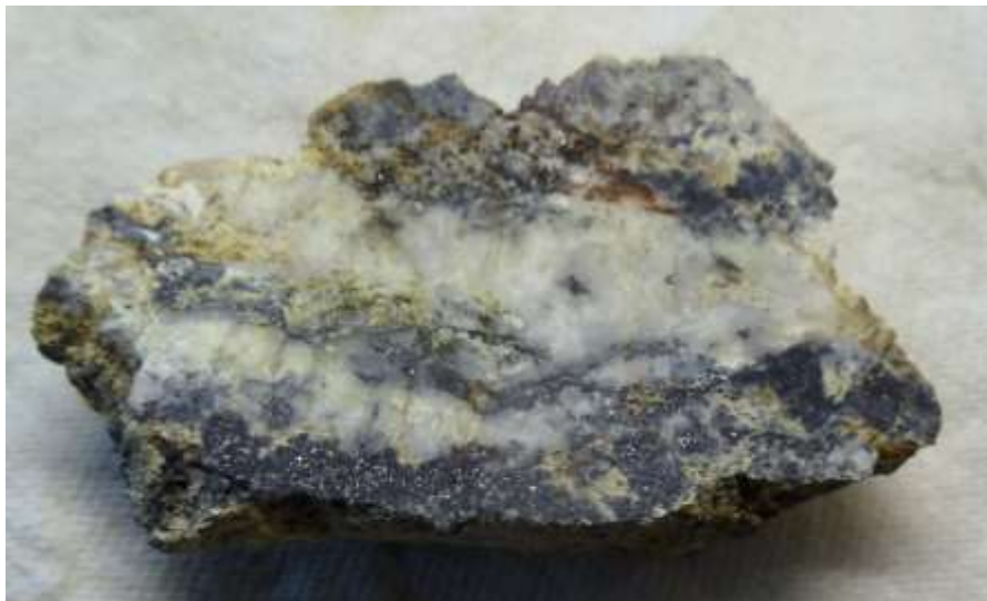
Figure 4: Banded Electrum and Silver Sulfosalts, Argenta Vein
