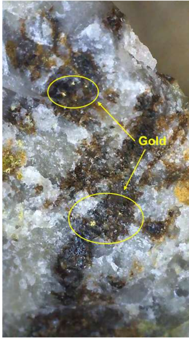
Figure 1: Two trench samples, including one pictured above, showed sphalerite-galena-chalcopyrite and native gold.
