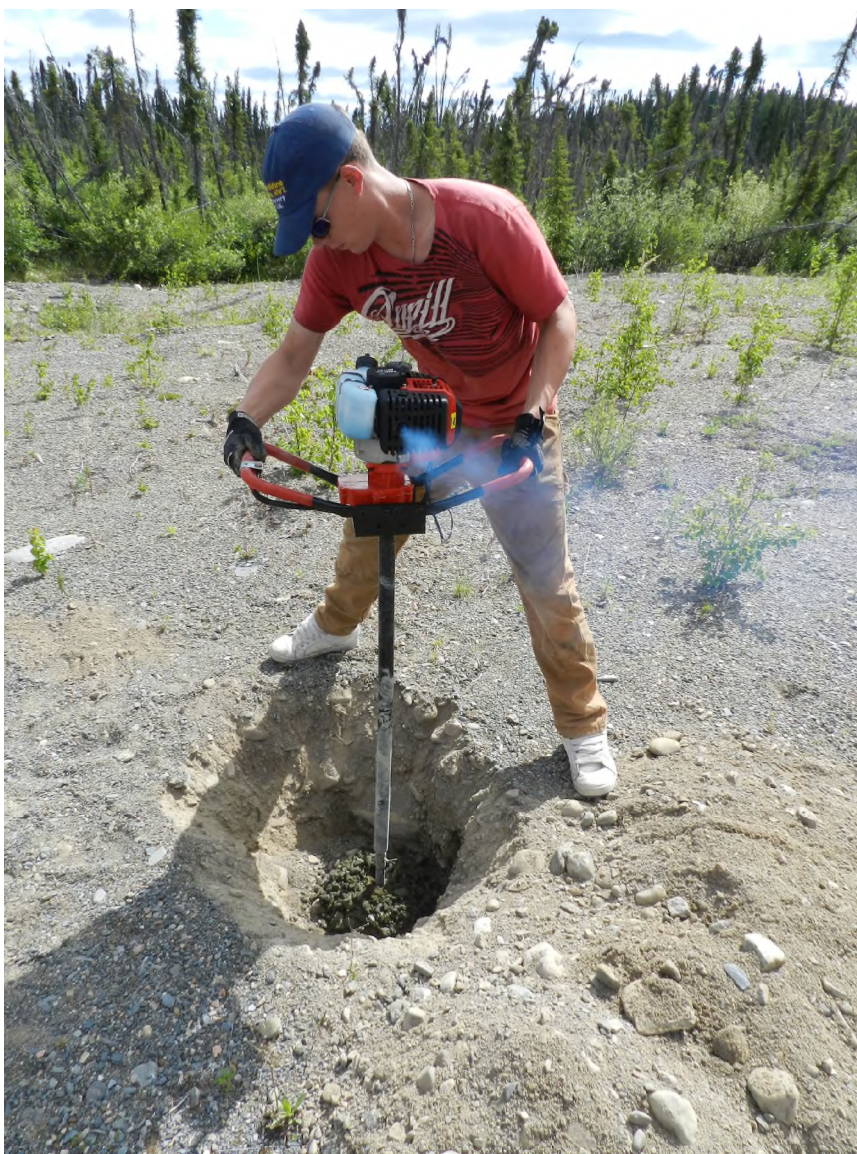
Photo 3. Auger sampling the Ger-Mac tailings pond in 2012.
