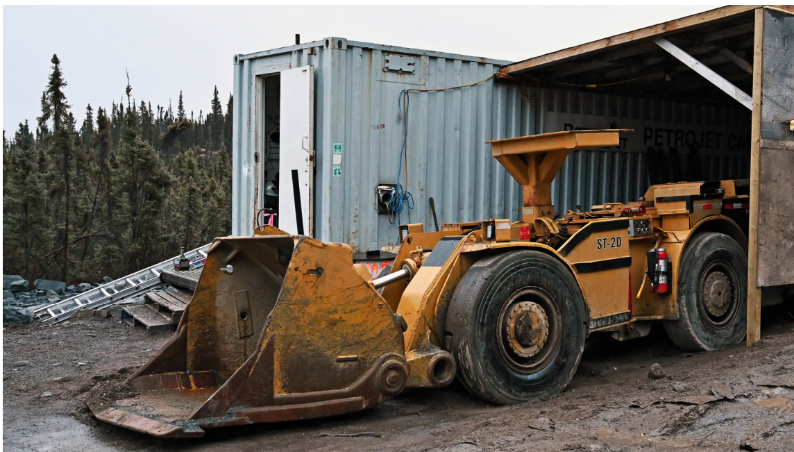
Photo 6. Two yard scooptram under cover for repairs.
