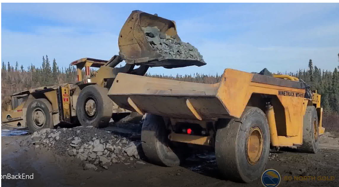
Photo 7. Scooptram loading 10 ton mine truck.
