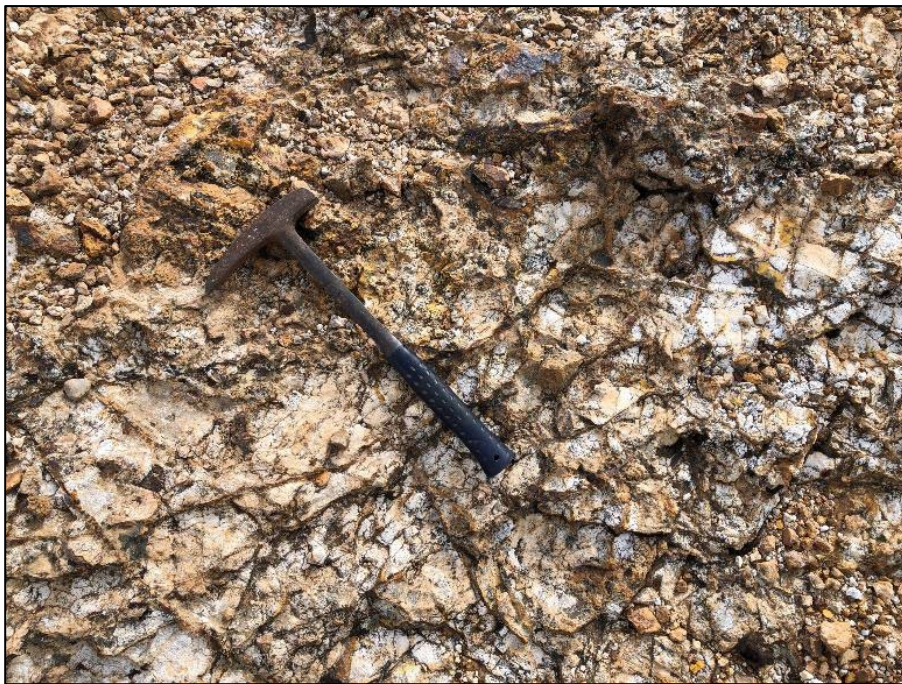
Figure 5: Outcrop from the Copper East target with intense porphyry related D-type veining anomalous in surface rock Cu geochemistry with grades of up to 108 ppm Cu.
