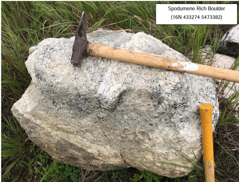
Figure 3: Spodumene bearing pegmatite boulder from the North Nipigon Project (Ontario Geological Survey AFRI 20000019444)
