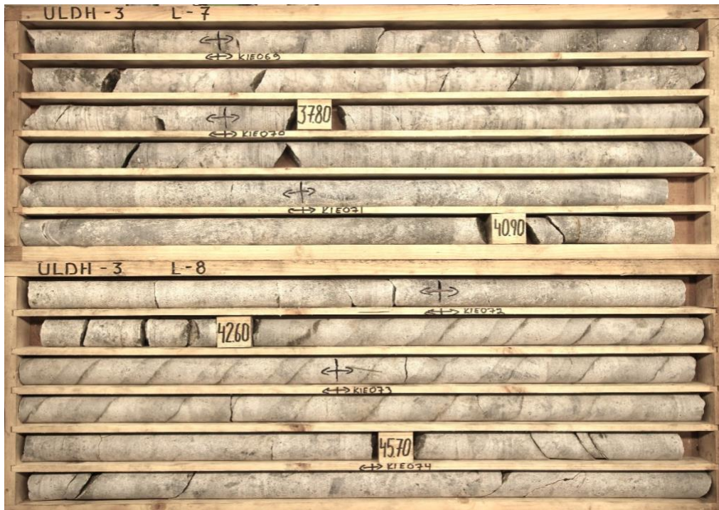
Drill hole ULDH-3 with pegmatite reporting 1.52% \text{Li}_2\text{O} over 25.95 m from 33.70 m depth down hole.
