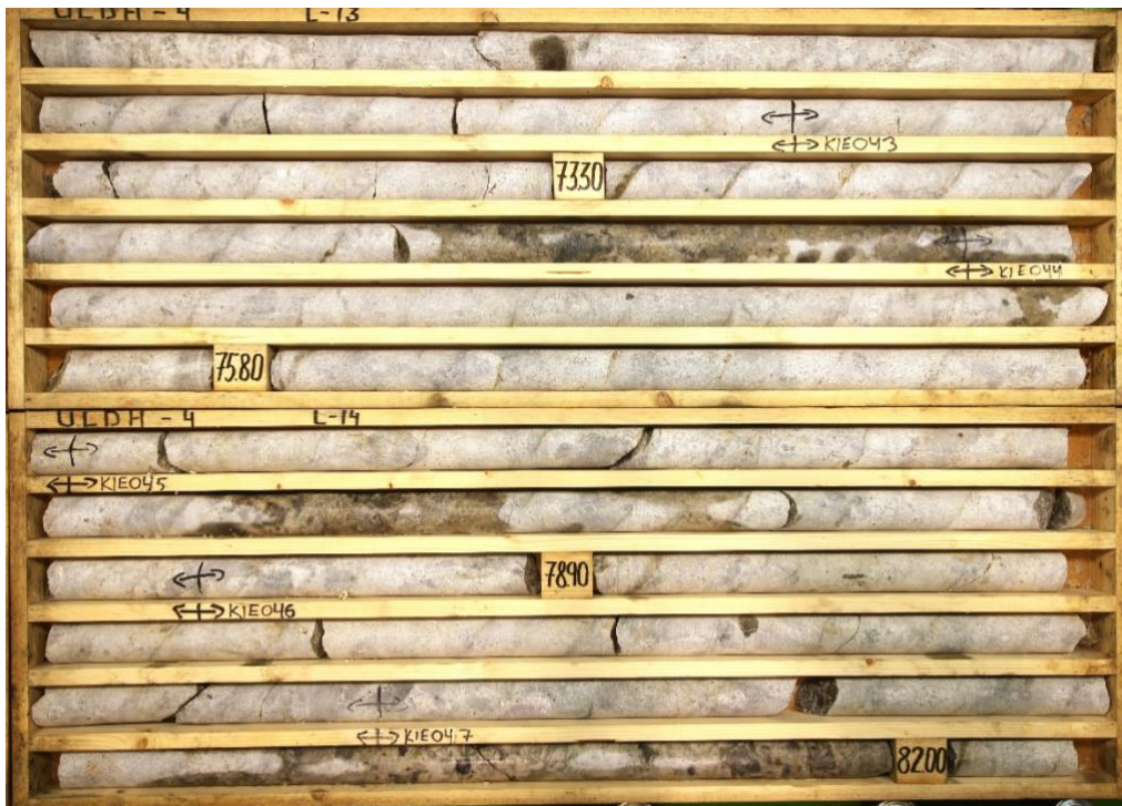
Drill hole ULDH-4 with pegmatite reporting 1.45% \text{Li}_2\text{O} over 29.50 m from 69.10 m depth down hole.
