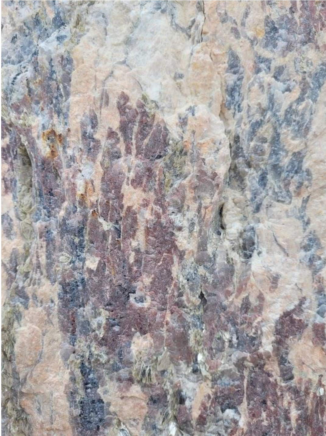
Photo 2 Biotite, quartz, and feldspar in enrichment zone in pegmatite, Liberty Lithium Project, South Dakota
