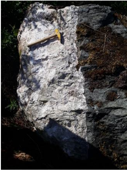
Figure 19: Coarse grained spodumene crystals and contact zone in a block
