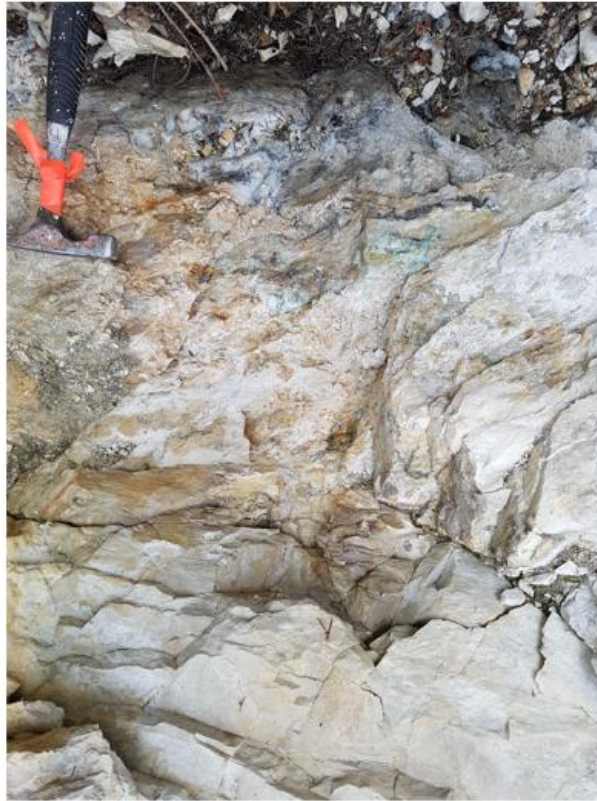
Photo 4: Contact Phyllitic Sequence and Limestone EBGs Member (Location Sample 102560).
