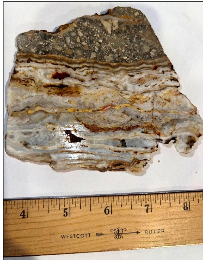
Figure 9: Nose Banded Vein in contact with Hydrothermal Breccia
