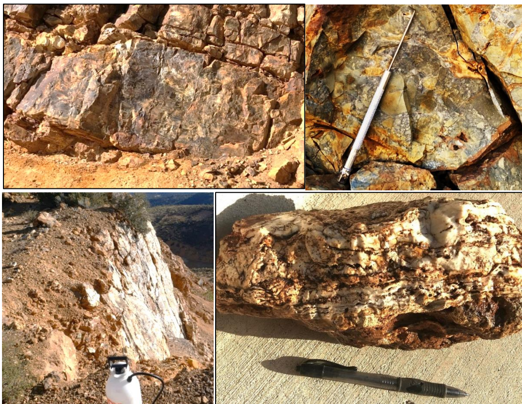
Upper left: pervasive silicification; upper right: hydrothermal breccia; lower left: epithermal vein viewed along strike; & lower right: crustiform banded vein.
