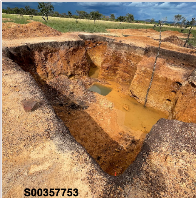
Figure 34 : Section through the Quaternary alluvial deposits at sample site S00357753 showing an iron-rich coarse-grained horizon underlain by dominant yellow brown sand and gravel. Photo JS.
