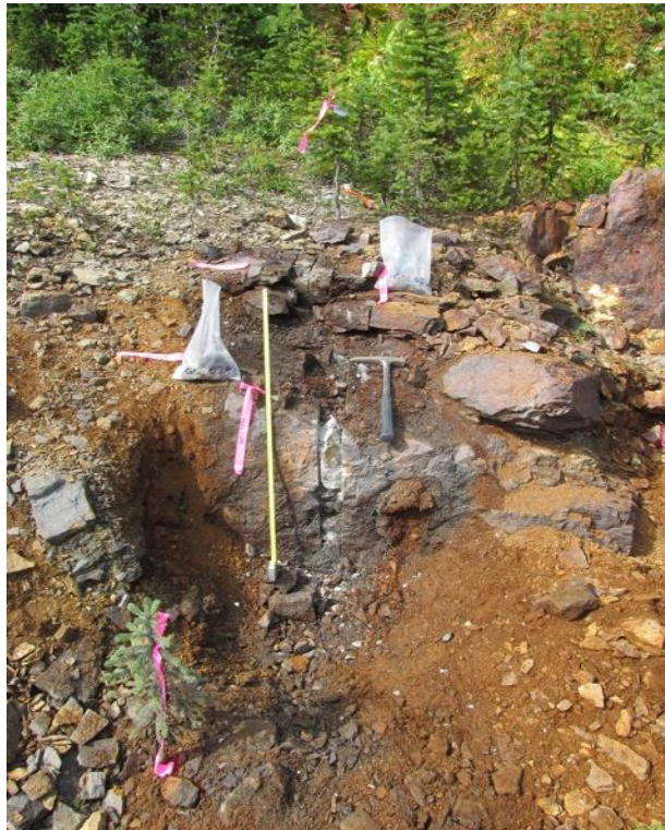
Photo 3. West Golden Eagle showing, diamond rock saw cut sample GOL-023, 22 centimetres interval length (435 ppm Cu, 4.02% Pb, 2.81% Zn, 50.9 ppm Ag, <100 ppb Au), and GOL-024, 42 centimetres interval length (265 ppm Cu, 852 ppm Pb, 368 ppm Zn, 6.4 ppm Ag, <100 ppb Au). Source: Kikauka, 2015.
