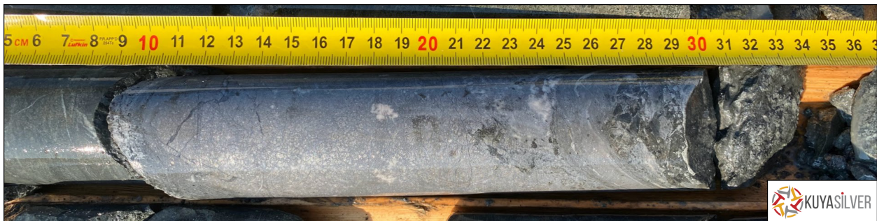
Figure 1: 0.19 m wide vein consisting of massive (ie. high concentration) cobalt and nickel arsenide minerals. The metallic grey vein material is a combination of cobaltite, skutterudite, and nickeline. This vein ranks among the widest, and is the highest-grade cobalt and nickel, that Kuya Silver has drilled to date at the Silver Kings Project. Vein was drilled in hole 24-SK-07 on the Hammerstrom fault, grading 29 g/t silver, 6.53% cobalt, 1.27% nickel (1833 AgEq*) over 0.40 m.
