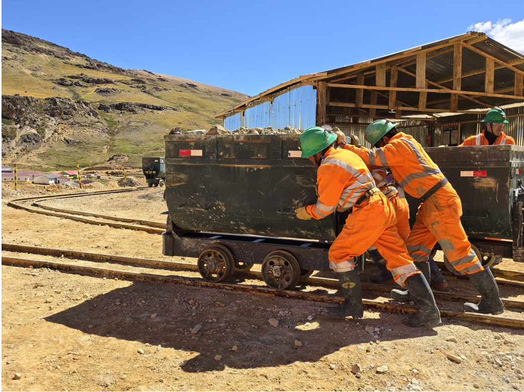
Figure 2: First full ore cart, material from the Española vein hauled up from the 640 level by a motorized winch and ready to be dumped on the ore stockpile
