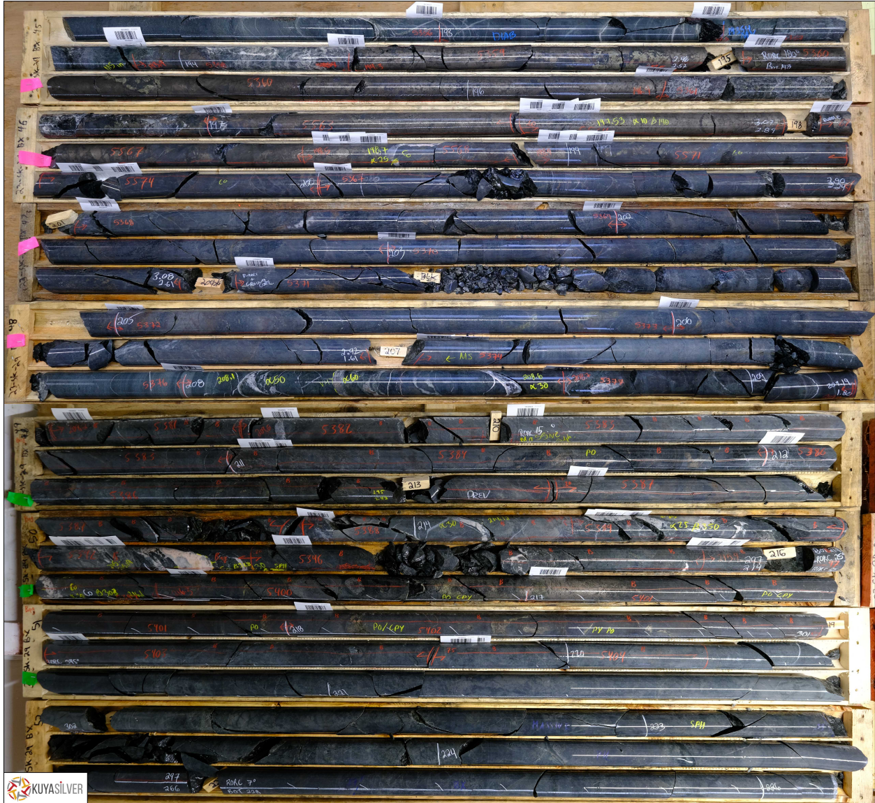
Figure 3: Photograph of semi-massive sulphide zone from hole 23-SK-29, which intersected highly anomalous silver (36 g/t), cobalt (0.04%), arsenic (0.10%), copper (0.31%), nickel (0.05%) lead (1.37%) and zinc (1.25%) over 23.10 m from 193.90 m on the Campbell-Crawford property. Local mineralized veins grade up to 131 g/t silver and up to 0.24% cobalt. This style of mineralization was recognized adjacent to economically viable mineralized veins at the nearby Beaver-Timiskaming Mine, which produced 19.2 million ounces of silver and 340,000 pounds of cobalt (Sergiades 1968).
