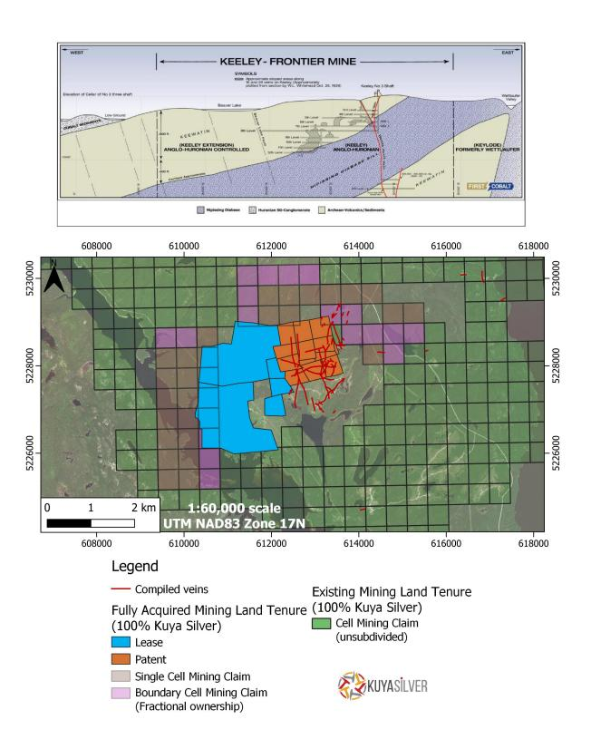
Figure 1: Map of the Silver Centre mining area, Cobalt mining camp, Ontario, including the updated property position and compiled veins from the Keeley and Frontier mines. An east-west vertical section of the Keeley Mine, showing the relative position of mineralization to the Nipissing Diabase sill, is included. Significant potential for further mineralization exists above the sill to the west and below the sill.
