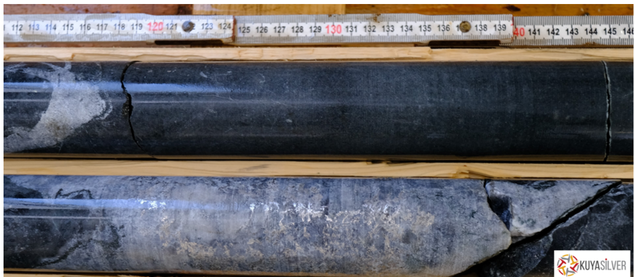
Figure 1: Metallic silver mineralization in newly-drilled core, Campbell-Crawford area of the Silver Kings Project.
