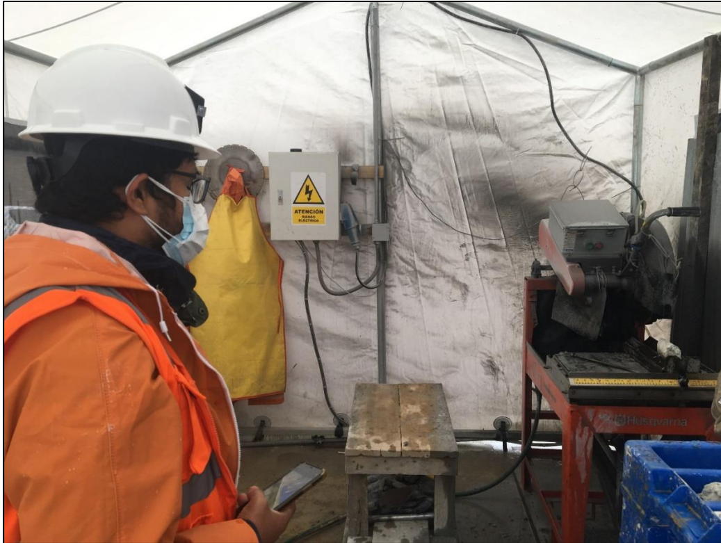
Figure 11-1: The on-site core cutting operation, completed by the geological service providers, BISA. (source: Simon Mortimer, 2021).
