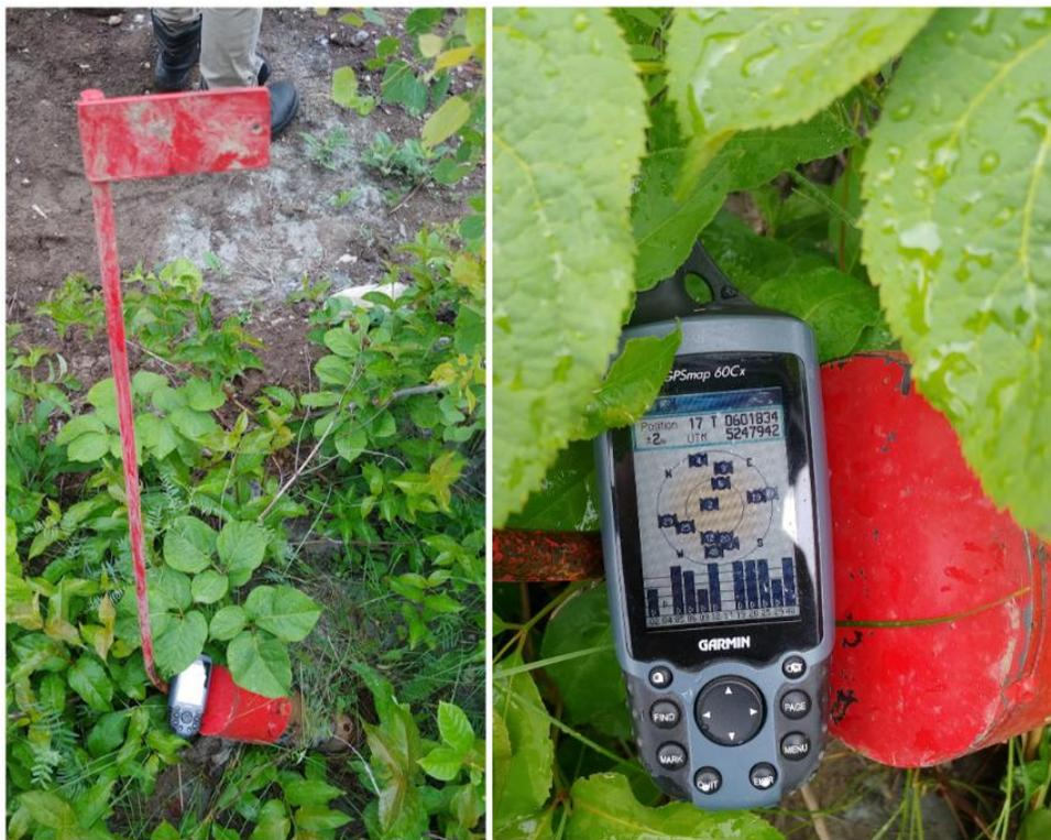
**Figure 12.3 – Casing of 21-KERR-001 verified during the site visit with coordinates in UTM NAD83, Zone 17**
