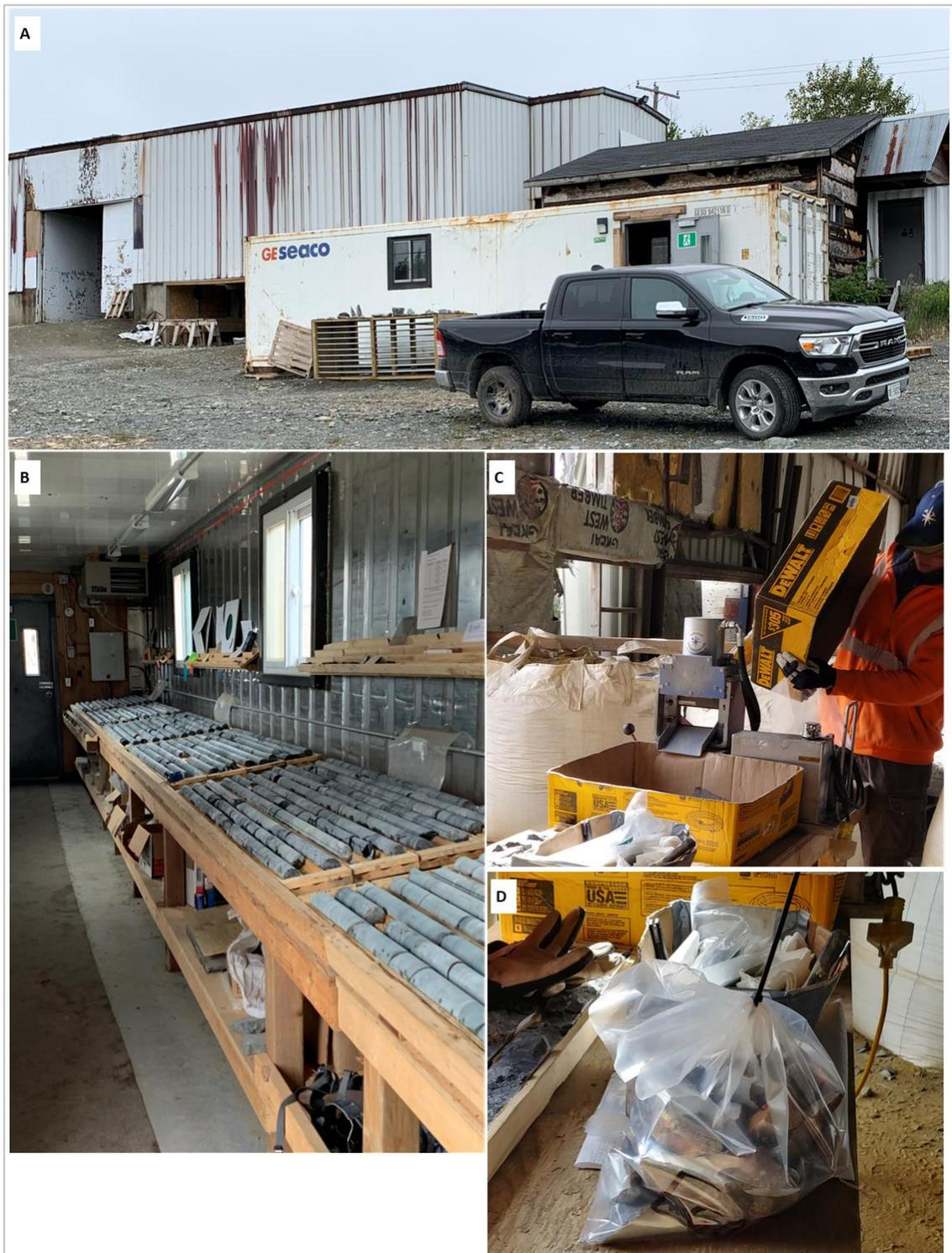
**Figure 12.1 – A) warehouse and core-logging facility at the Canadaka Mill site; B) indoor logging facility; C) core-splitting in progress; D) sample ready to be shipped to AGAT for analysis.**
