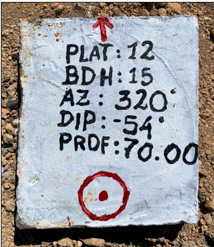
Figure 10-3. Example of cement marker/hole cover with drill hole information placed at each of the drill hole collar locations (source: Kuya Silver, 2021).
