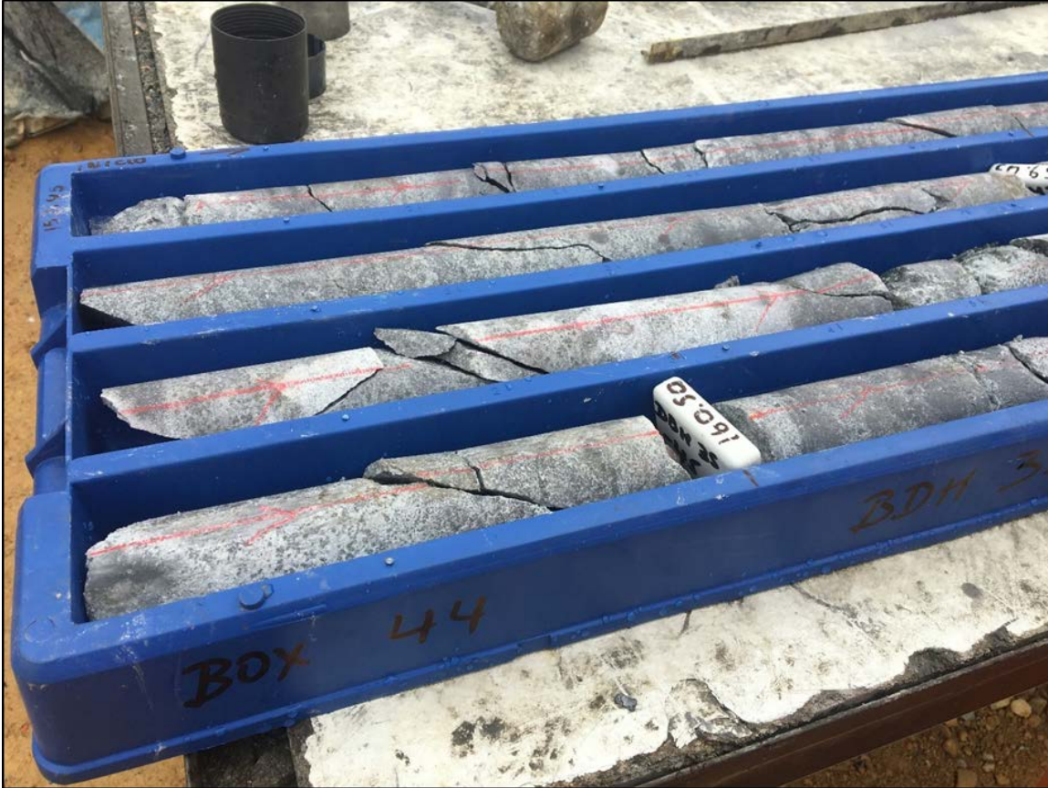
Figure 10-5. Orientated drill core measured using the Devico orientation tools, recorded by the drilling contractors, Ingeomin (source: Simon Mortimer, 2021).
