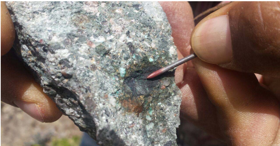
Igneous clast from dike containing abundant copper oxide (blue material) and native copper. The "nail test" is a common field tool to identify copper.
