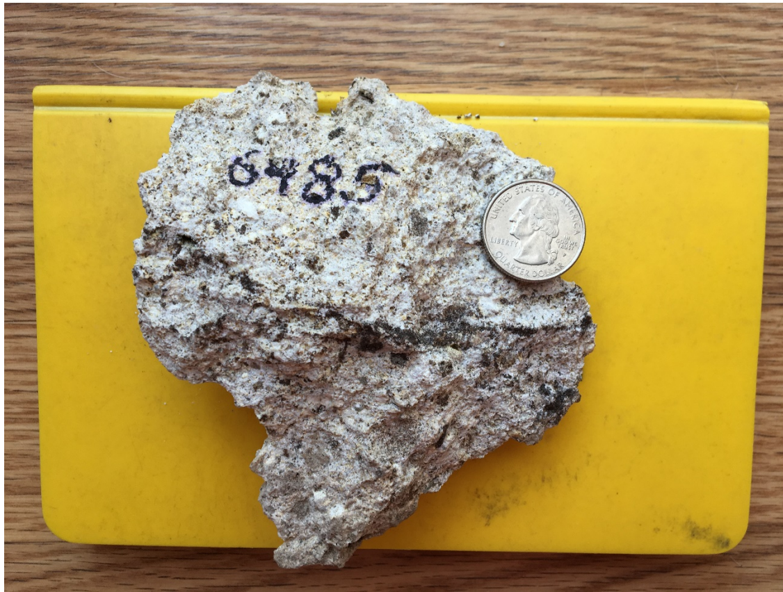
Figure 14 of the Technical Report. Diatreme breccia from Base Outcrop, author's sample 6485: 1.25 g/t Au, 6.3 g/t Ag. Note irregular veinlets marked with MnO. Coin diameter = 2.43 cm
