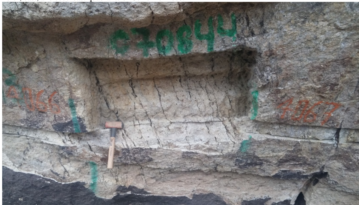
Figure 17 of the Technical Report. Box and channel samples by Standard Silver from Base Outcrop. Channel sample 70840: 2m @ 3.77 g/t Au. Sheeted, irregular veining with Feox-MnO, minor quartz.
