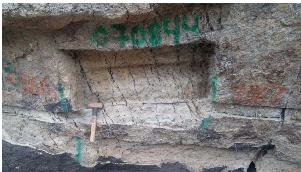
Figure 17. Box and channel samples by Standard Silver from Base Outcrop. Channel sample 70840: 2m @ 3.77 g/t Au. Sheeted, irregular veining with Feox-MnO, minor quartz.
