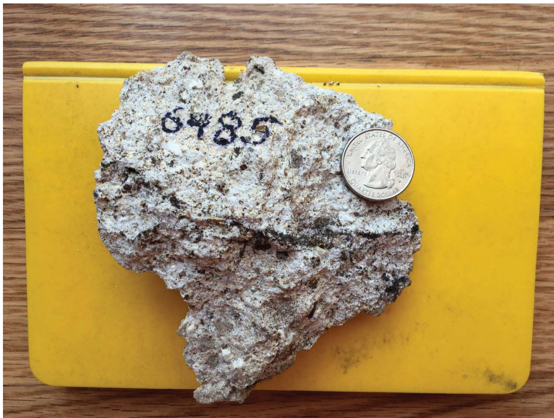
Figure 14. Diatreme breccia from Base Outcrop, author's sample 6485: 1.25 g/t Au, 6.3 g/t Ag. Note irregular veinlets marked with MnO. Coin diameter = 2.43 cm
