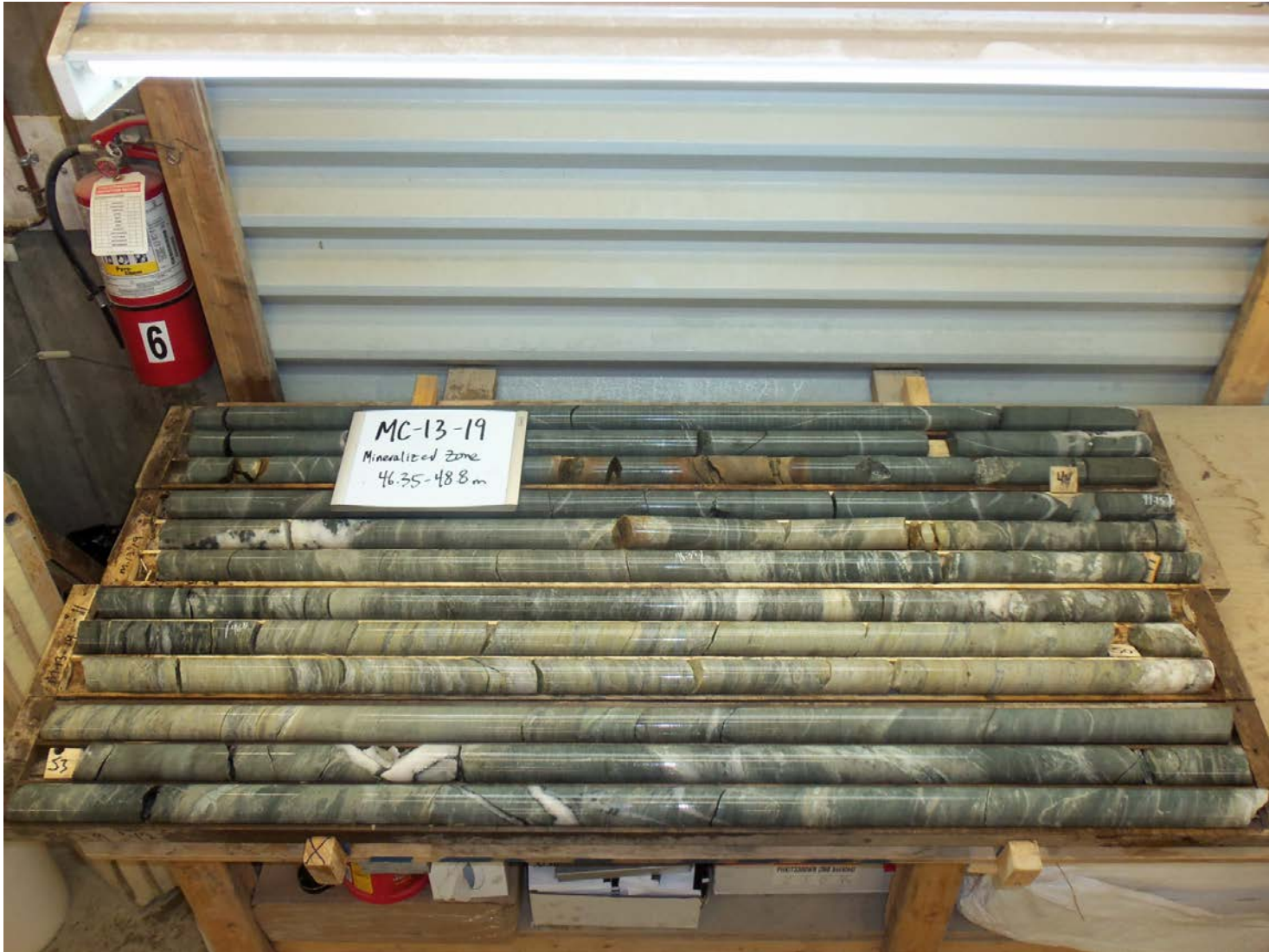
Figure 11: Photograph of mineralized zone in MC-13-19 showing the presence of white-coloured quartz veining within the pyritized shear zone.
