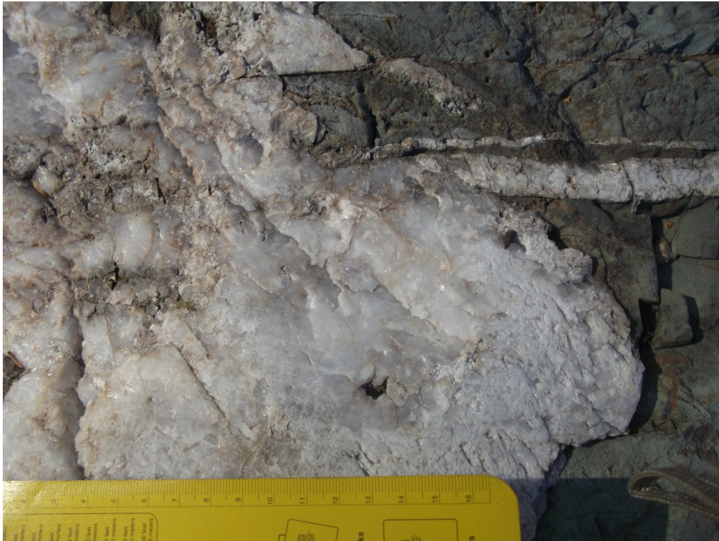
Figure 6: Picture from above showing relationship between 020 veins and flat lying veins in Stripped Area 7.
