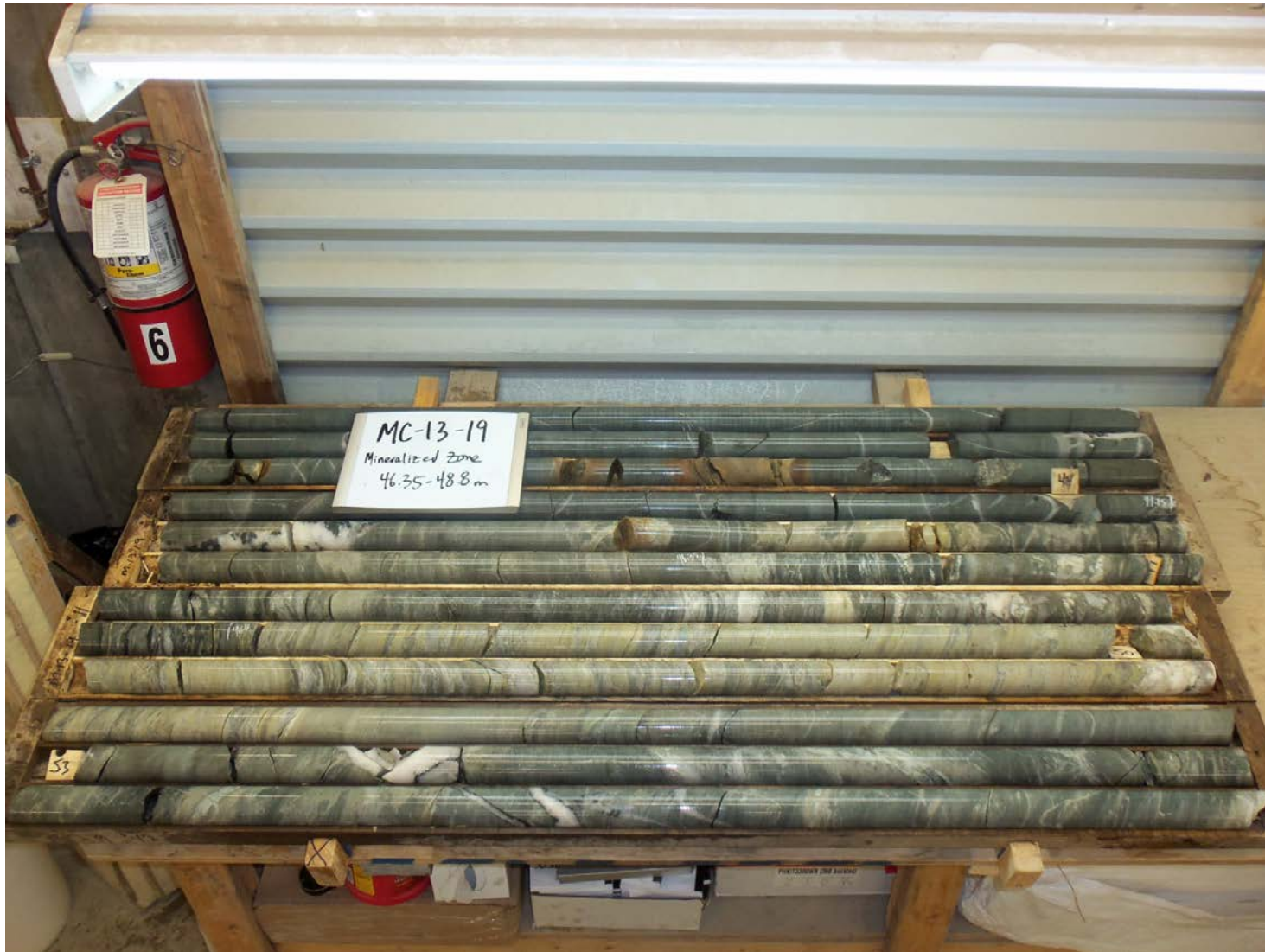
Figure 12: Photograph of mineralized zone in MC-13-19 showing the presence of white-coloured quartz veining within the pyritized shear zone.
