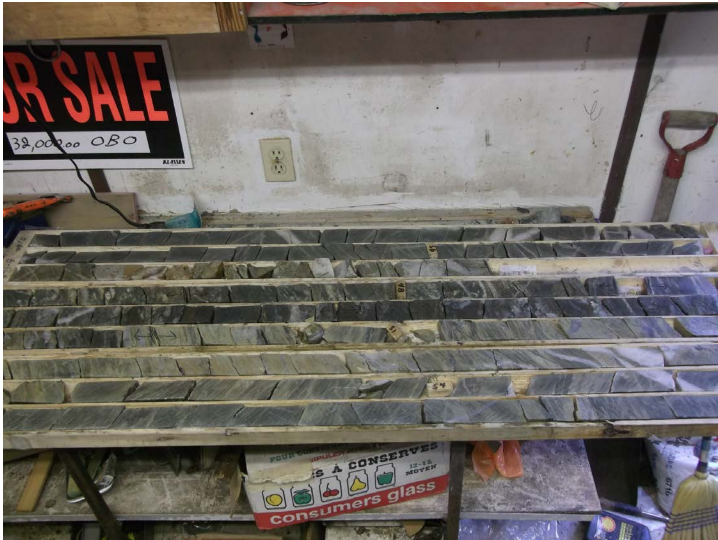
Figure 11: Photograph of the mineralized zone in MC-11-04. Area of missing core contained the highest assay value and is reported to be a large white coloured quartz vein.
