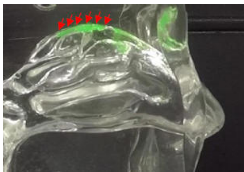
Figure 3b Sol-gel spray profile gels and coats olfactory epithelia (inhalation model, cast temperature 34 °C).
