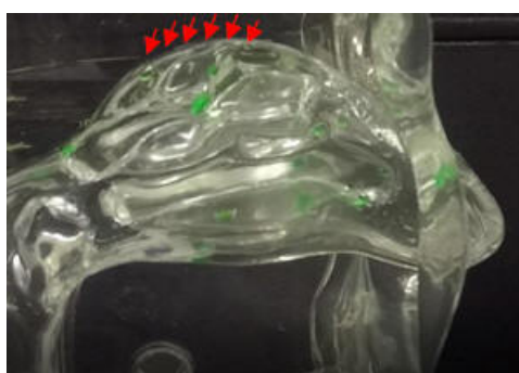
Figure 3a Liquid spray generates a random droplet profile (inhalation model, cast temperature 34 °C).
