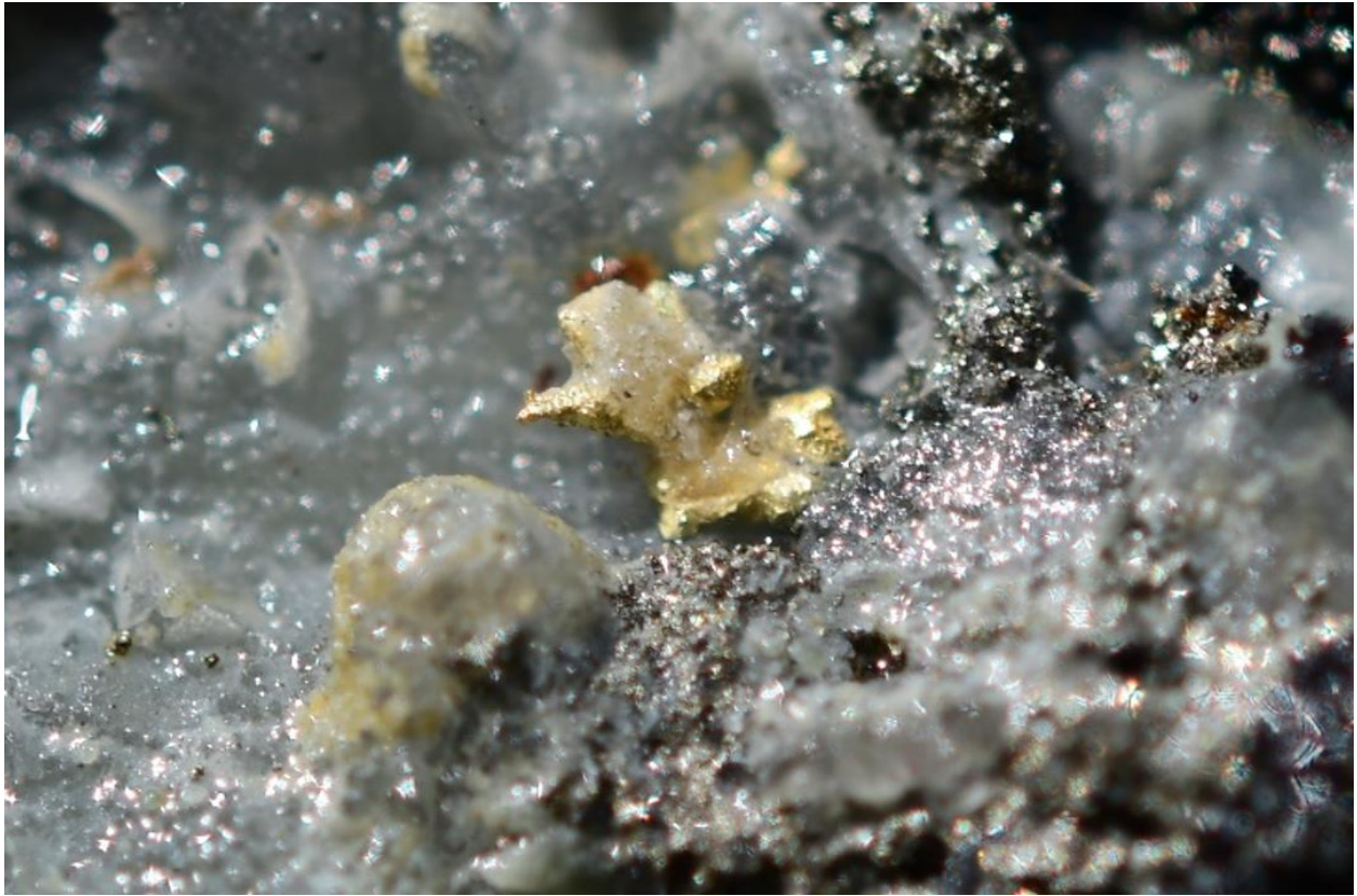
(Figure 2 – Close-up of coarse visible gold particle in Figure 1. Width of picture frame is 7mm.)
