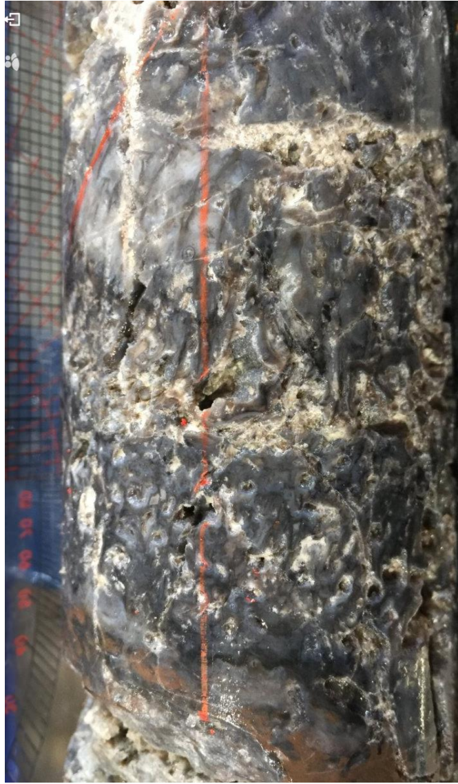
(Figure 2: Fibrous columnar algal remains, now silicified, occurring within a bed of sinter in core. Down hole depth is 314 m.)
