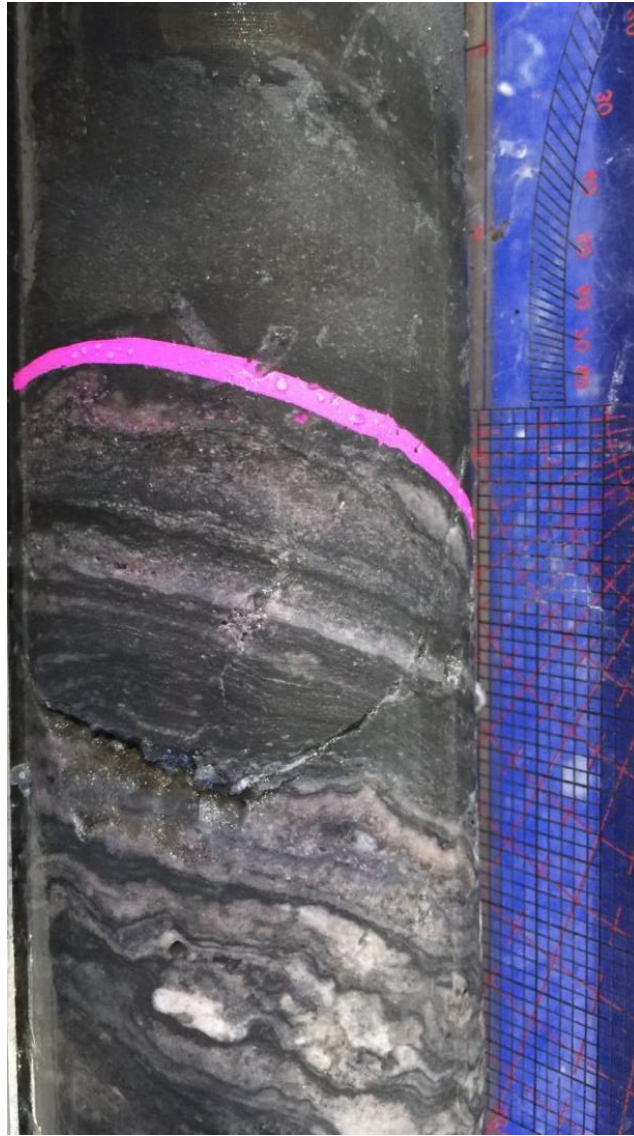
(Figure 1: Laminated gray and white hot spring silica sinter overlain by dark gray silty mudstone in core. Dark coloration partially originates from fine sulfide mineralization. Down hole depth is 303.8 m.)
