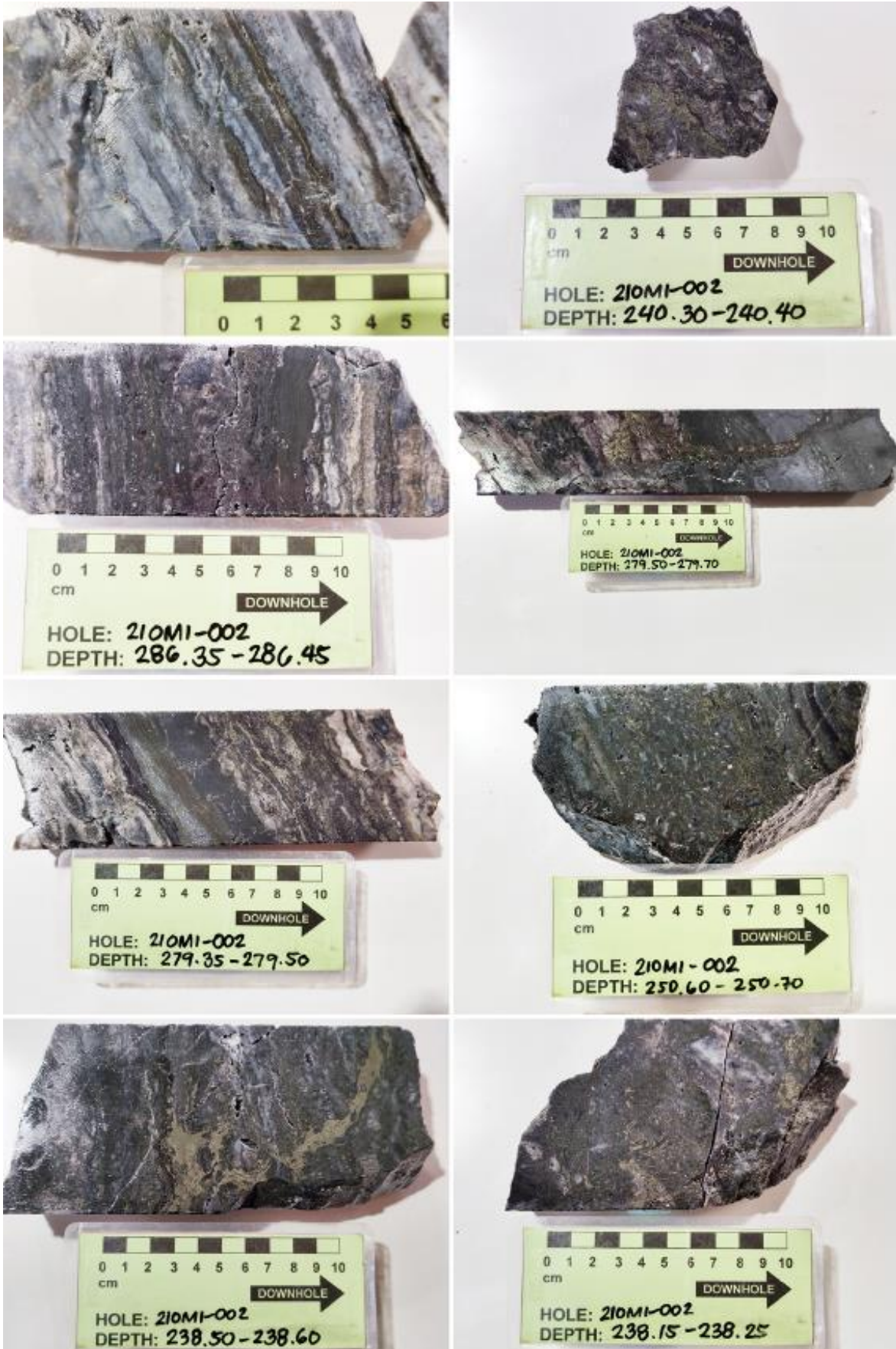
(Figure 3: Examples of sulfide rich sinter from various intervals in hole 210MI-002. Brassy and gray material is pyrite. Light gray, white and tan areas are silica.)
