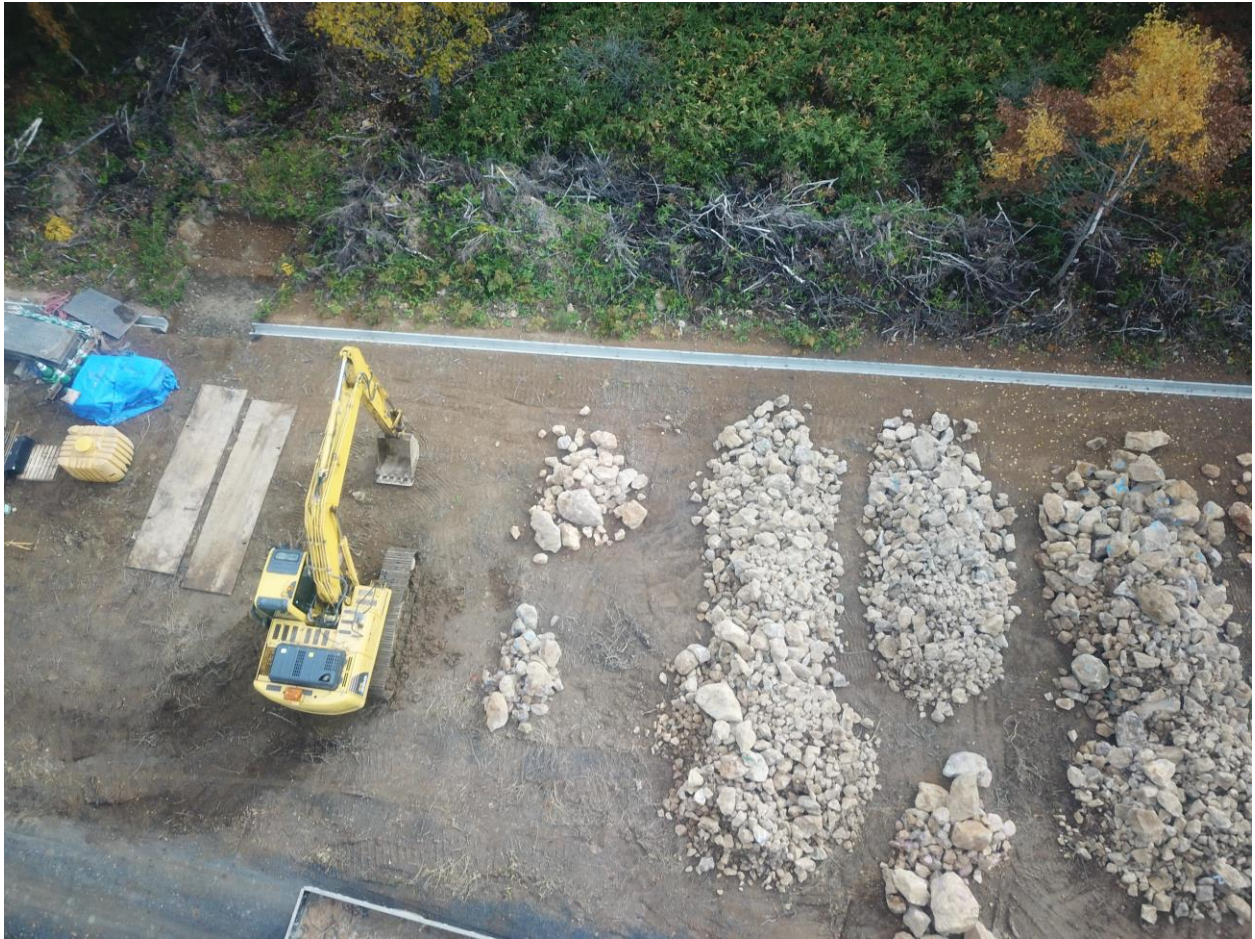
(Figure 6: Aerial image of stockpiles of vein material recently collected from trenches at Omui Mine site. More material will be added to this in 2020 and shipped to a Japanese smelter.)
