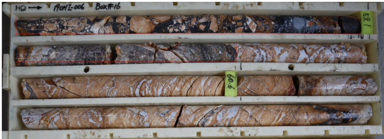
(Figure 4: Vein intercept (red line) in hole 190MI-006 drilled at Omui Mine site. This interval displays brecciation along with local patches of silver sulfosalts and electrum.)
