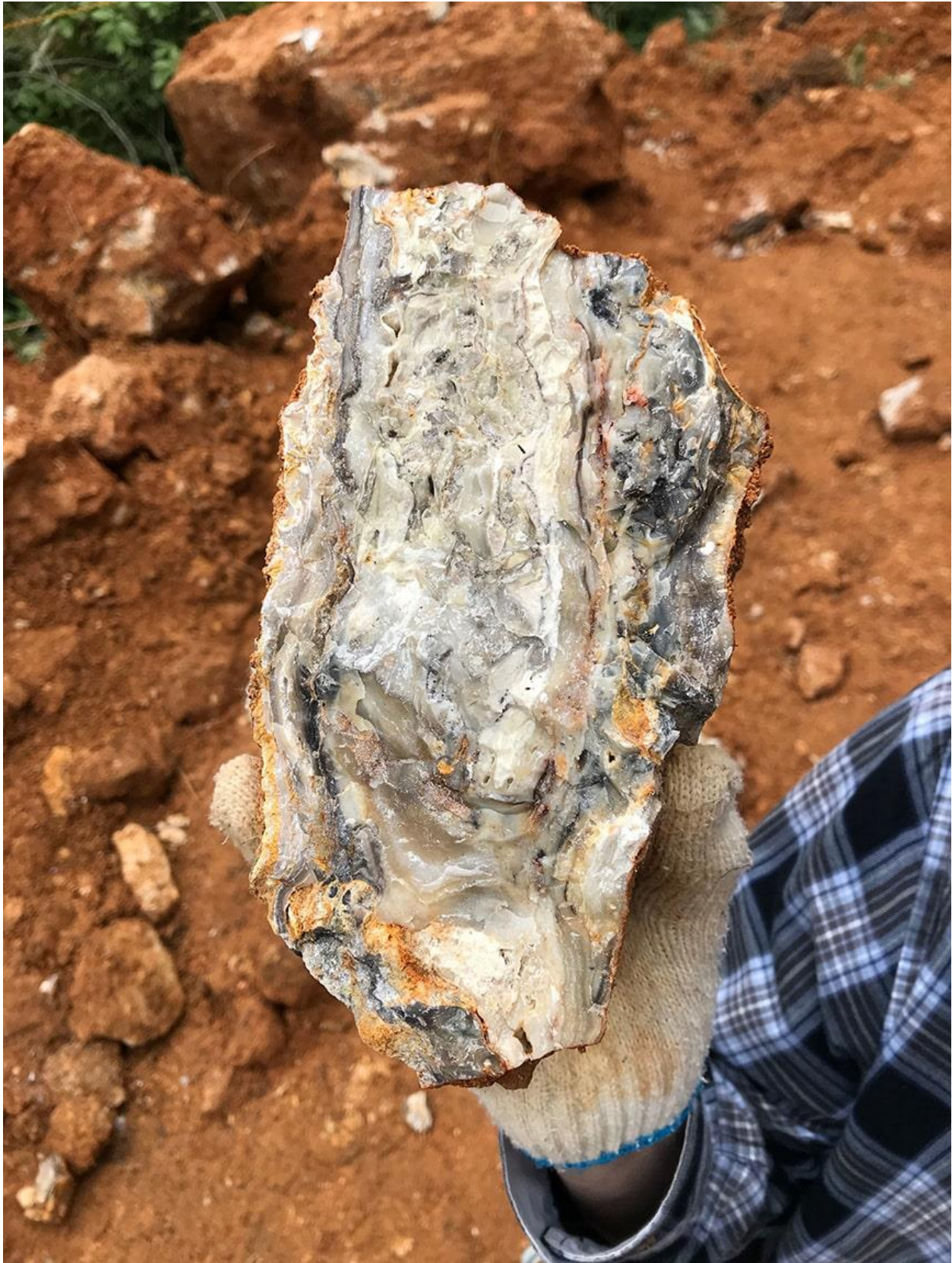
(Figure 5: Sample of vein material from a 1.5 m wide exposure of the N. Honpi vein recently exposed in trenching. The outcrop that was exposed is approximately 20 m long.)
