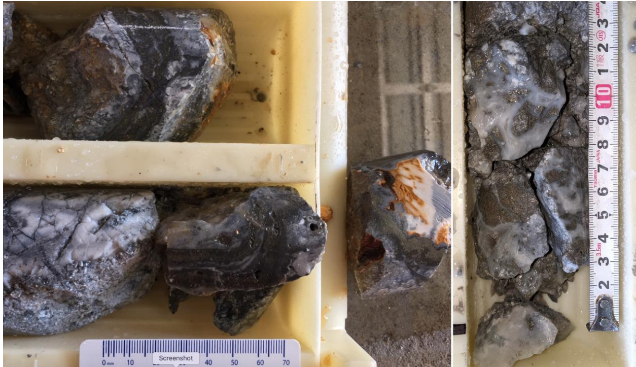
(Figure 4: Banded quartz veins encountered in hole 19OMS-004. These veins displays notable pyrite and marcasite like the high-grade vein encountered in hole 19OMS-002. Assays are awaited.)
