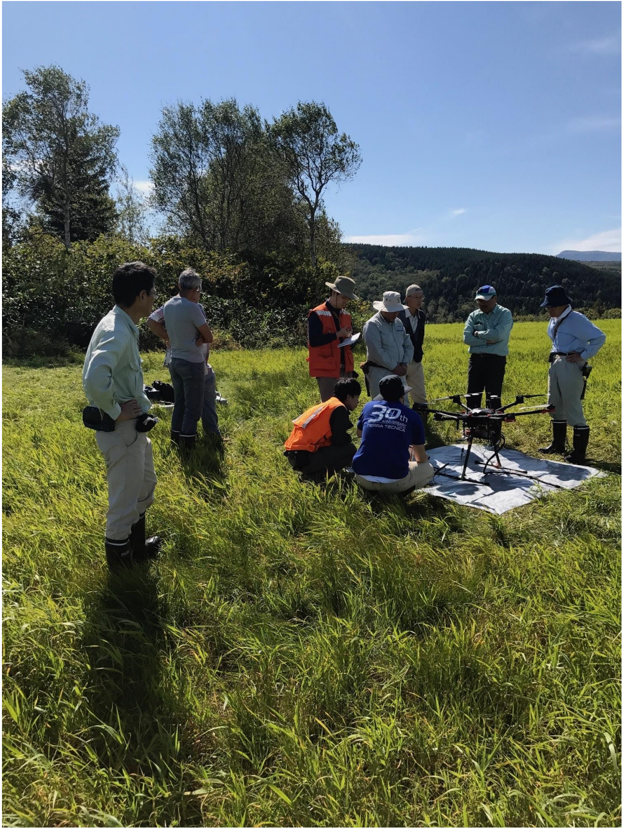
(Figure 2: Drone-based magnetic survey system)
