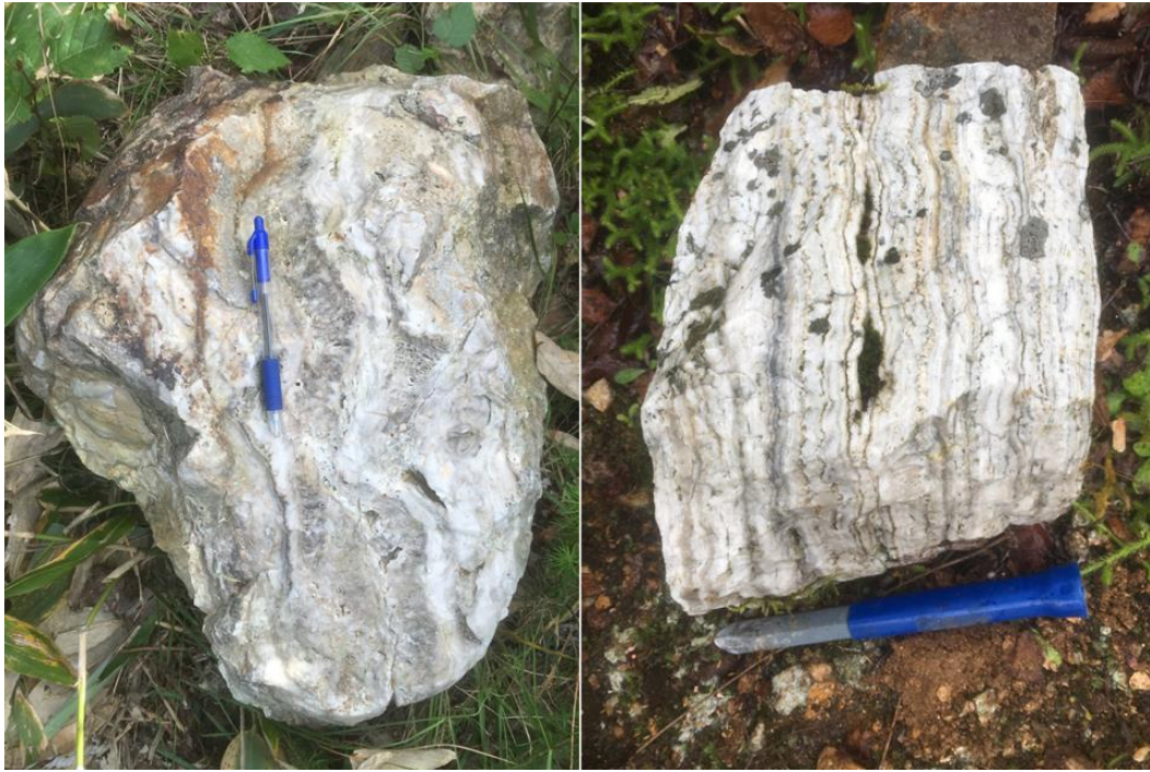
(Figure 1: Examples of banded epithermal quartz vein from Omui (left) and Hokuryu (right) mines. Finely bladed textures along some bands are silica pseudomorphs after bladed calcite, an indicator of boiling in the hydrothermal system.)
