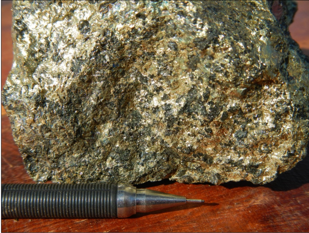
Figure 6-10: Sulphide mineralisation from the Tambi open-cut workings.
