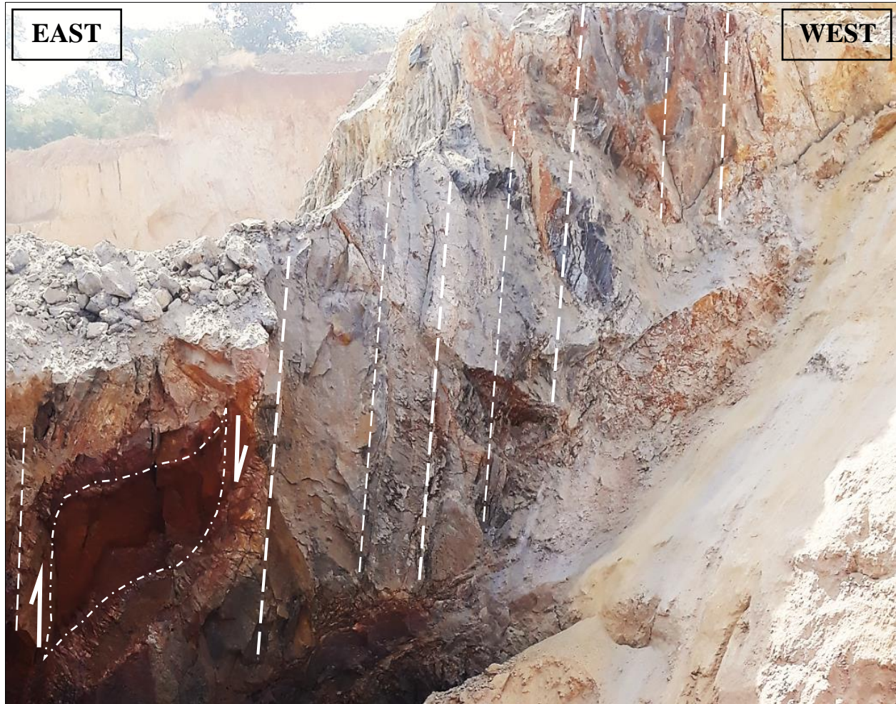
Figure 25.4: Photograph of the Mamadouya Shear Zone in vertical section (Looking toward the south) showing the steeply easterly-dipping shear zone that affects highly mineralized turbidite sequence composed of alternating sandstone and siltstone. The Shear zone is concordant and shows typical kinematic indicator such as S-shaped Sigmoidal structure within the sandstone layer that indicates a reverse displacement during deformation. (Photo taken during December 2020 site visit)
