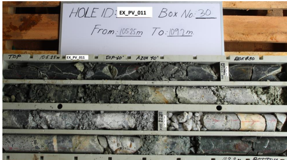
Figure 2: Significant epithermal vein intercepted in EX PV 011, which returned 0.4m grading 0.83 g/t Au and 0.15 % Cu
