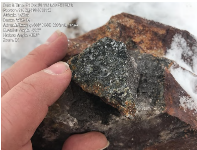
Figure 0.12 (as shown above) - Example of a sample observed by the Author – fracture controlled sulphides (arsenopyrite – pyrite – chalcopyrite).
