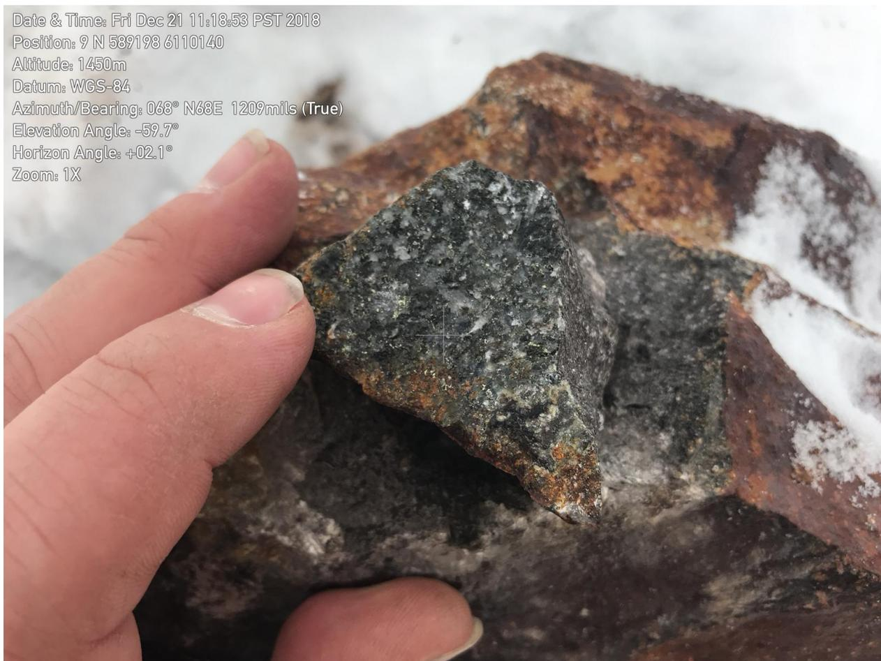
Figure 12.1 Example of a sample observed by the Author – fracture controlled sulphides (arsenopyrite – pyrite – chalcopyrite).
