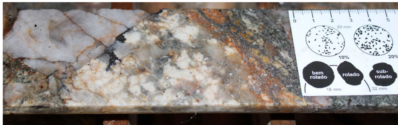
Photograph 8.1: Black Wolframite surrounding Quartz Fragment in Santa Helena Breccia
