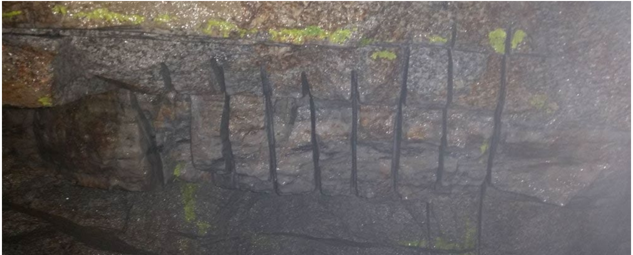
Photograph 9.2: Vein Sampling Cuts across Sample Br_01 (Minerália, 2020)
