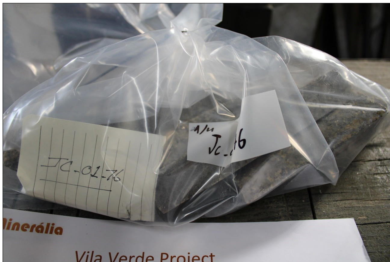
Photograph 11.2: Verification Sample JC_01_76 of Quarter-Cut Drill Core
