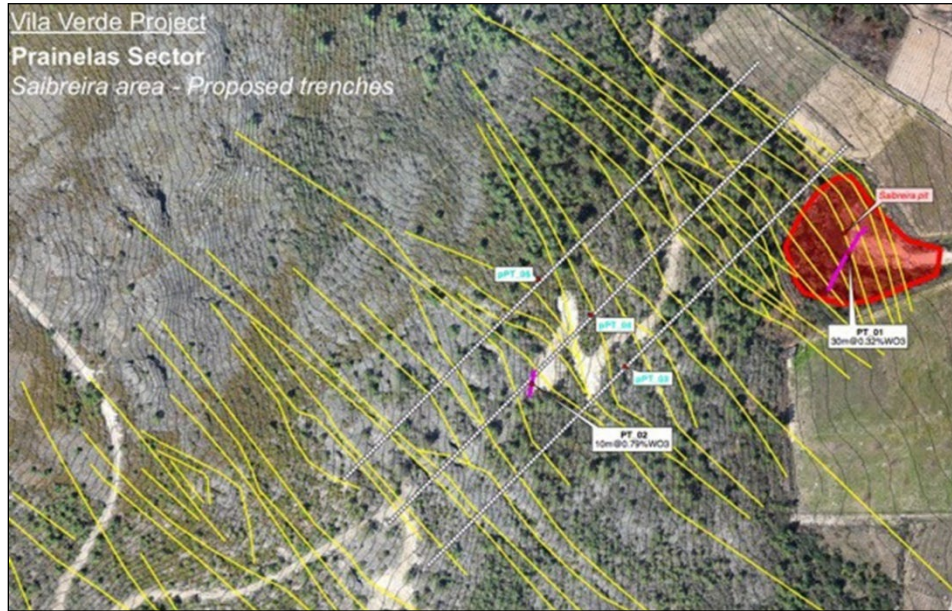
Figure 9.3: View of the Prainelas Sampled Trenches (magenta) and Proposed Trenches (cyan) (Minerália, 2020)
