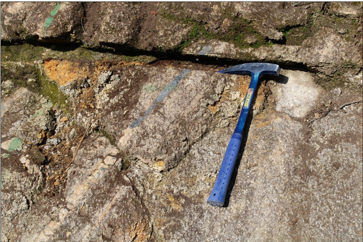
Photograph 7.7: Lens of Wolframite (blue-grey colour) in a Quartz Vein at the Prainelas Zone
