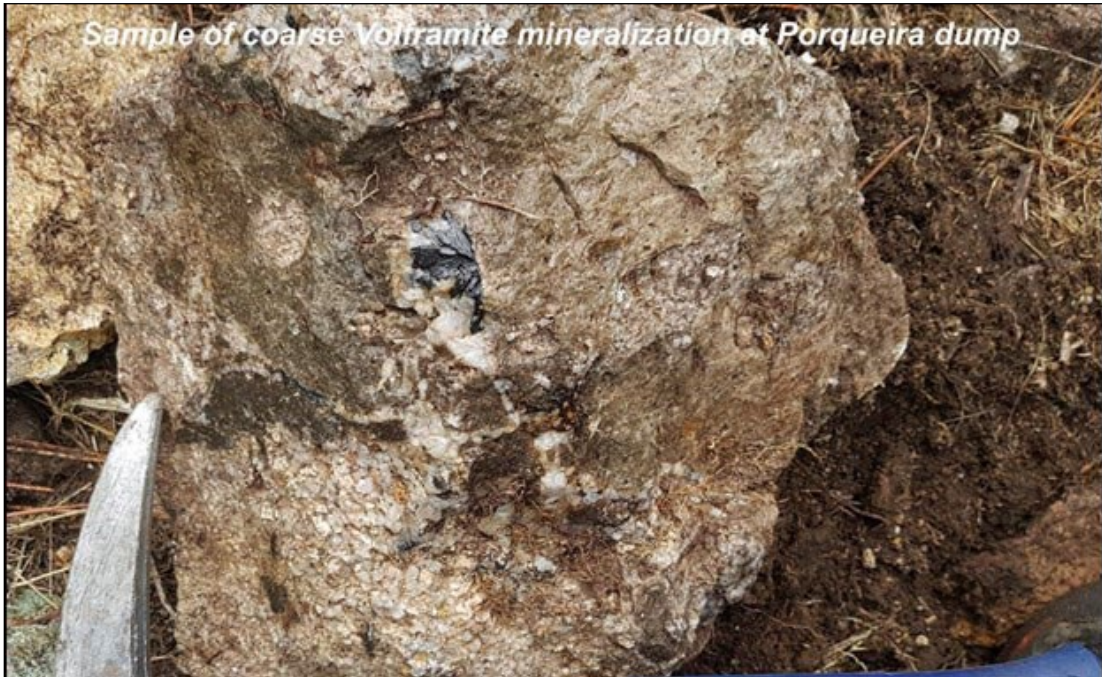
Photograph 9.7: Wolframite in Altered Granite, Porqueira Waste Dump (Minerália, 2020)
