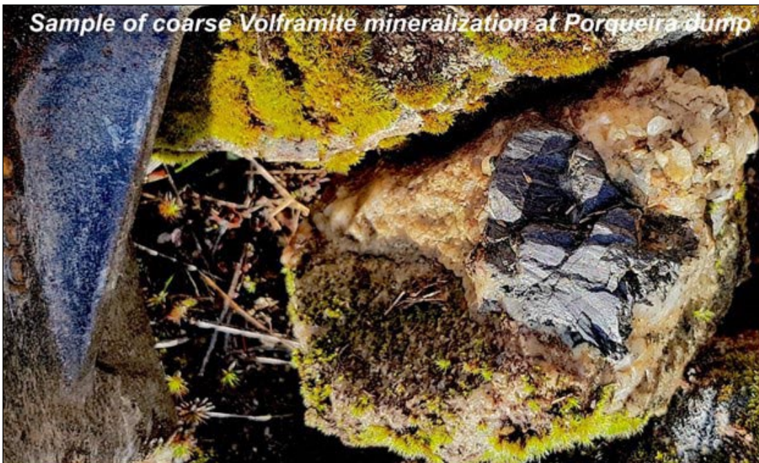
Photograph 9.8: Coarse Wolframite at Porqueira Waste Dump (Minerália, 2020)
