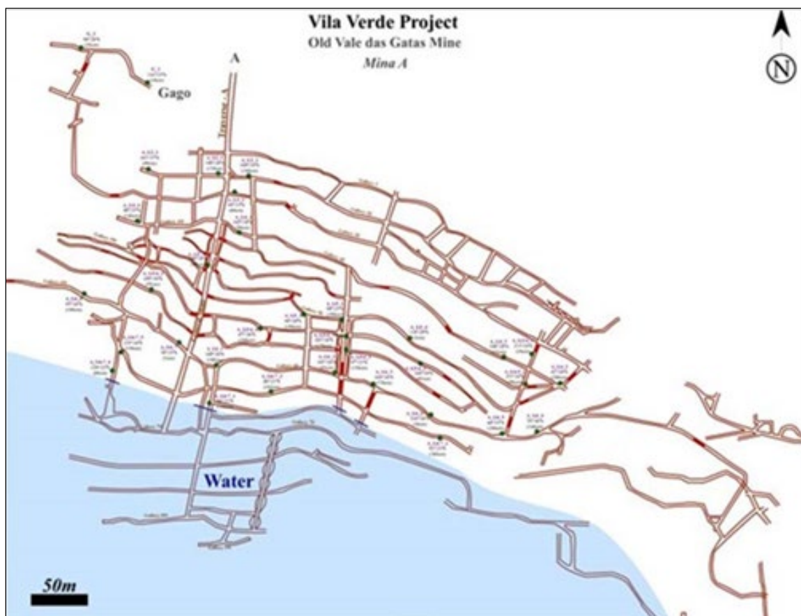
Figure 6.2: Underground Workings of the Vale das Gatas Mine (Minerália, 2020)
