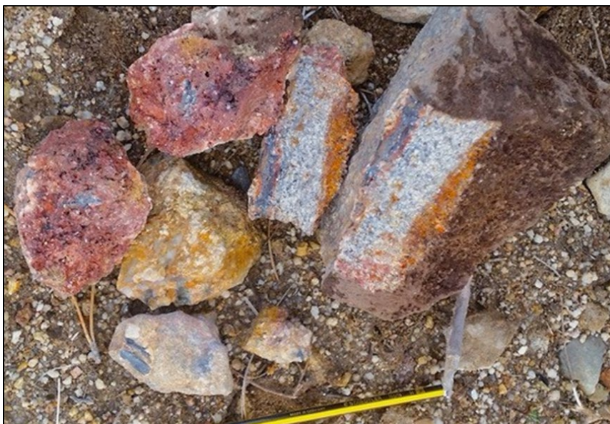
Photograph 7.10: Greisenized Granite with Quartz-Wolframite Veinlets and Disseminations (Minerália, 2020)
