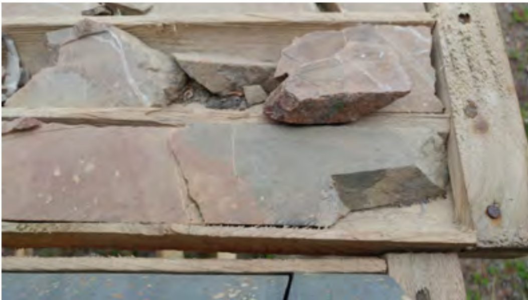
PICTURE No 10: Sharp contact between alterations in a basaltic lava flow. The basaltic rock is hematized and weakly potassic (red to bron) or chloritized (green). Hole TP-04-07.
