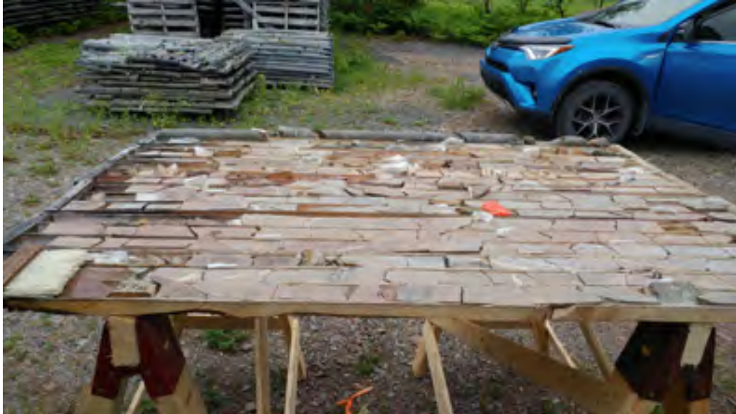
PICTURE No 8: Beginning of hole TP-04-07. Altered zone (silicified and hematized, presence of stockwork). The core has been sawed, sampled and assayed. Gold assay up to 1.72 g/T over 1 m.
