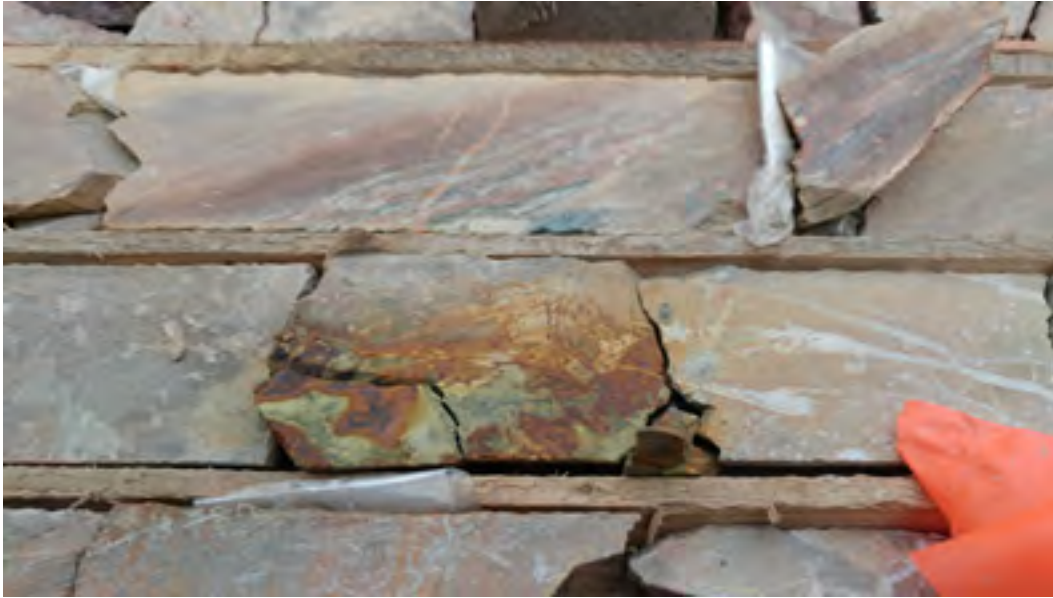
PICTURE No 9: Altered sulphide in hole TP-04-07. Typical arsenopyrite weathering.
