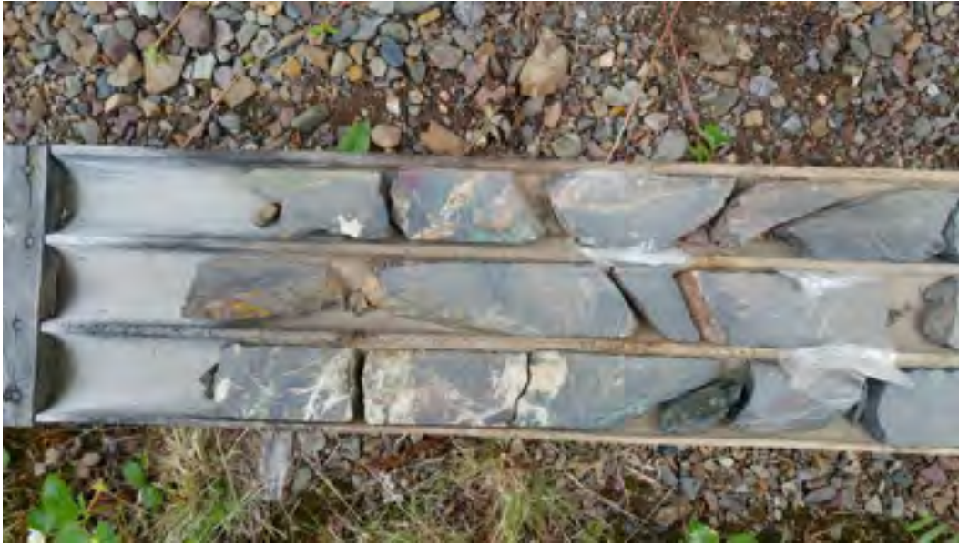
PICTURE No 7: Zone of stockwork in altered basalt, Hole TP-04-07.
