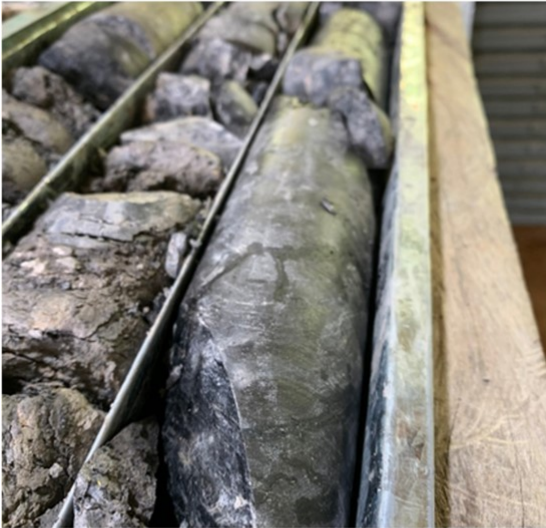
Figure 3 - Core sample showing coal deposit
