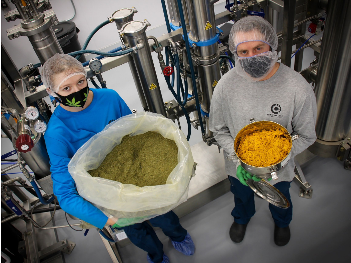
Two members of CLC's extraction team hold dried biomass (left) and crude oil (right) in front of the Company's Vitalis R-200 CO2 extraction machine
