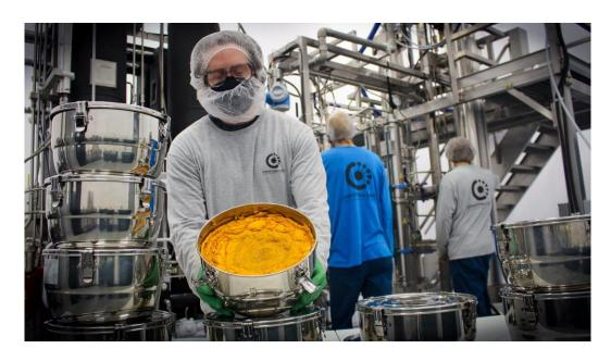
A vessel of crude oil weighing approximately 5 kg / 11 lb is held by a CLC extraction team member, showing the distinct golden hue of wax which will be removed in the distillation process, resulting in a finished oil product with a viscosity and colour similar to honey.
