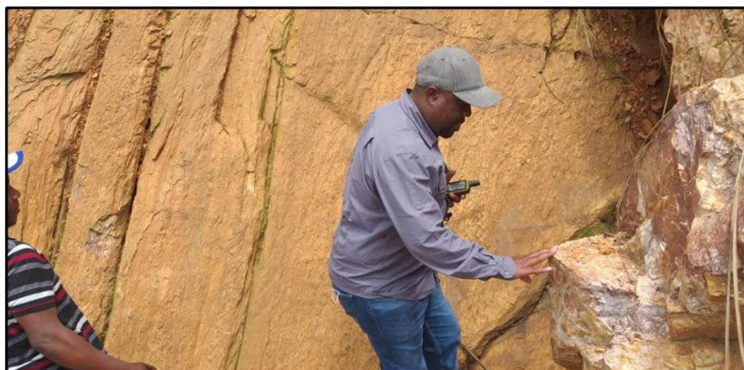
Figure 12-5. Quartz vein overlaying conglomerate from Akyanga ridge which is currently being mined by the artisanal miners.
